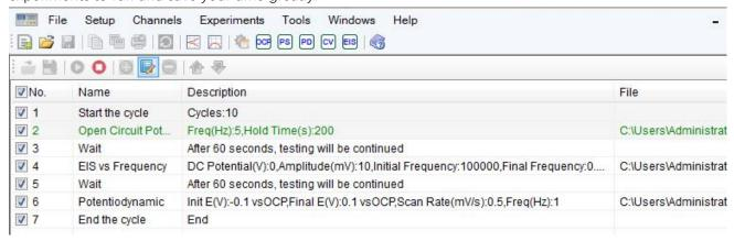
Data open: You can open the data files by txt format in notepad. Data can also be opened in Origin
