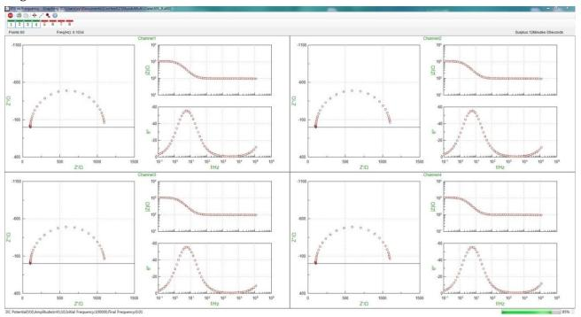
You can also choose different experiment in each channel. Set the parameters for each experiment, and run each experiment independently.
