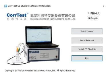
(3) For potentiostat more than one channel, we use Ethernet communication. So there is no need to install drivers. Firstly, install the .net 3.5. If your computer has already
