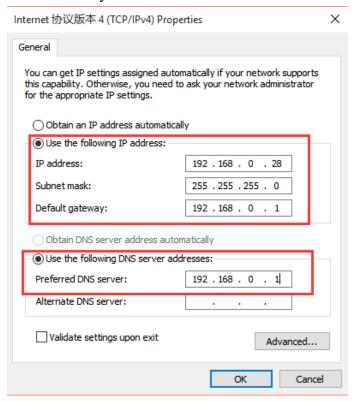
(5) Open CS Studio5 software, "Setup" → Connection → "Ethernet" → Manual
