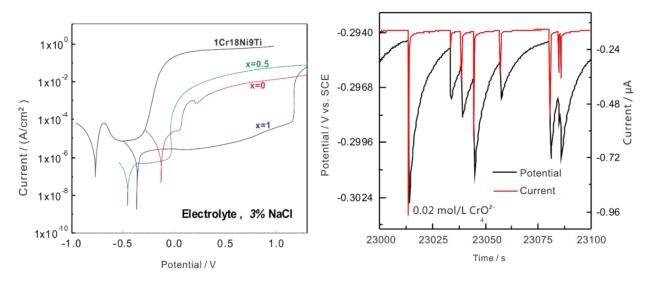
Polarization curves of Ti-alloy& stainless steel in 3%NaCl solution(left) EN of low-carbon steel in 0.05mol/LCl+0.1mol/LNaHCO3(right)
